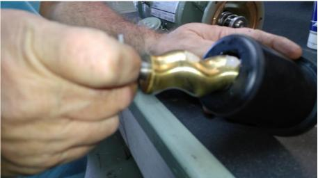
DO NOT GET SILICONE ON LIP OF STATOR – It is a good Idea to wipe lip off rubbing Alcohol or equal product. Seal must be clean and dry.
