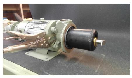
Step 4. (after nose cone / housing is removed) – the (150) stator and portion of Rotor with T-Bar cutter will be exposed.
