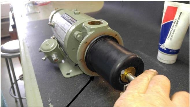
Stator Lip Seal in Housing.
