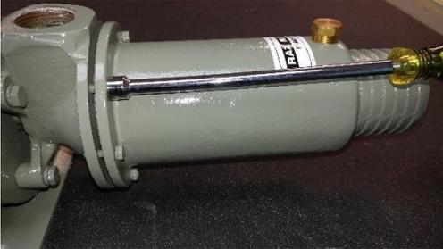
Step 4. (after nose cone / housing is removed) – the (150) stator and portion of Rotor with T-Bar cutter will be exposed.
