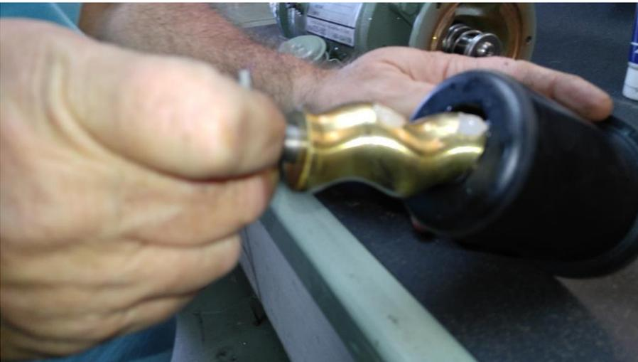
DO NOT GET SILICONE ON LIP OF STATOR – It is a good Idea to wipe lip off rubbing Alcohol or equal product. Seal must be clean and dry.
