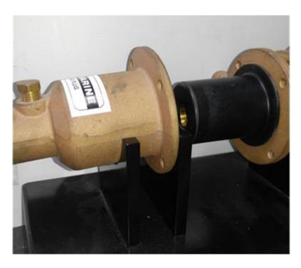
Step 4. After removal of stator insert new stator. It should fit nice and snug. Simply twist and push on. If it is too hard you may have wrong stator. There is a left hand and right hand stator. So if you have one on the boat make sure it is the correct one! Use Silicone lube or equal, do not use oil etc. Dish soap or even water is fine. You just want to prevent dry running during priming.
